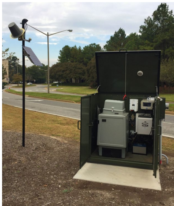
Figure 2. Ruggedized housing and components present at each stormwater monitoring station.
